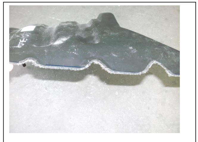
Figure 15: Liner looks like this after trimming
