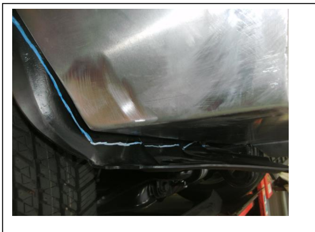
Figure 14: Marking liner to trim
